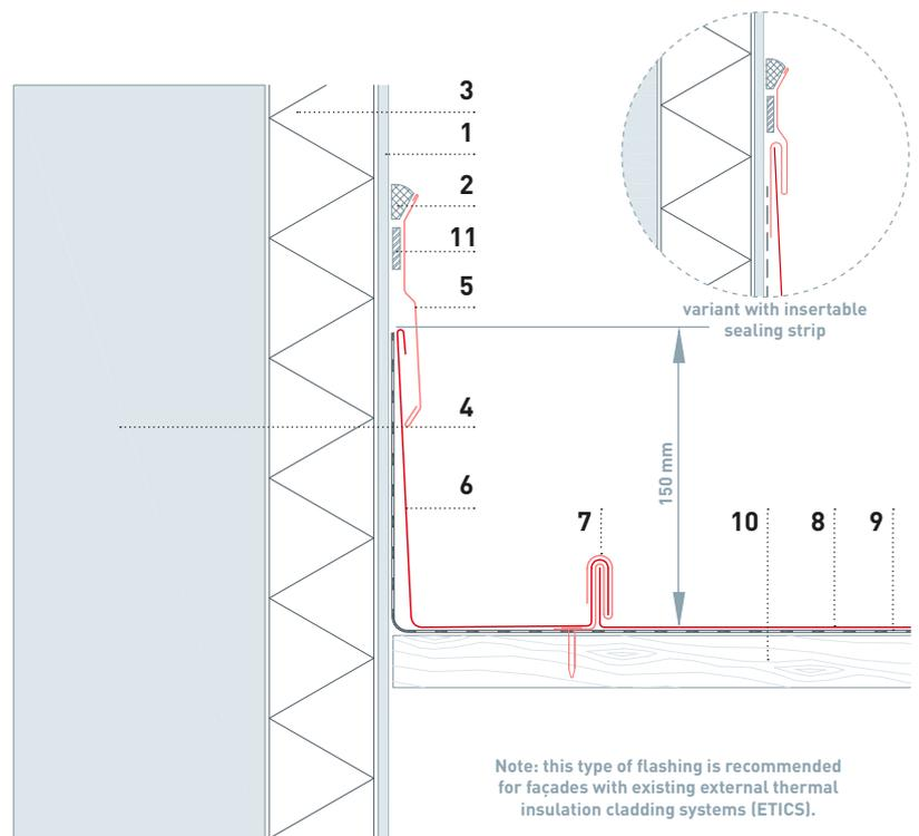
Note: this type of flashing is recommended for façades with existing external thermal insulation cladding systems (ETICS).
