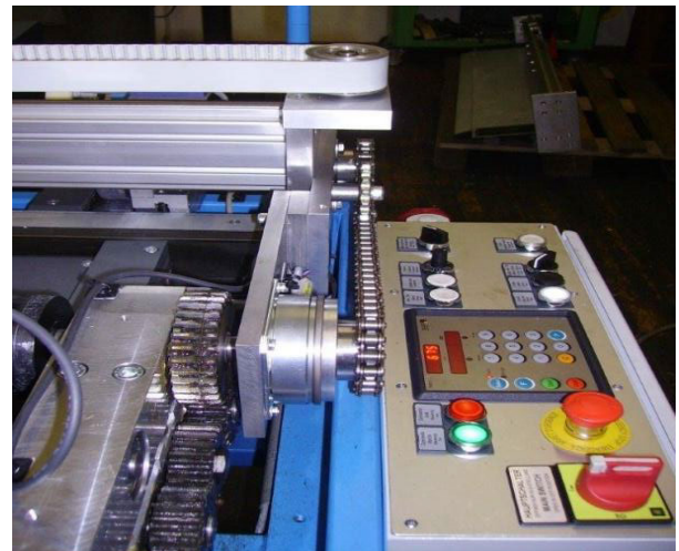
Control panel and electromagnetic clutch overview
